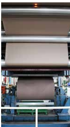
Finishing of the backing materials
